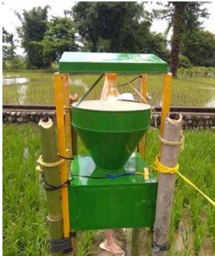
Figure 20. Light trap installed in a paddy field for hopper monitoring
